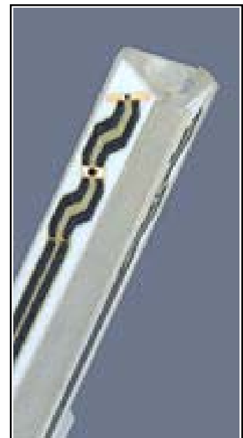
Inside View of ET3DV6 E-field Probe
