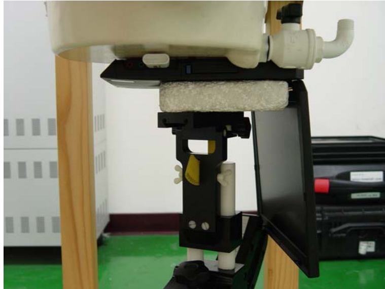
Fig. 9.5 IBM R31 Notebook Bottom Touch with Horizontal USB Port
