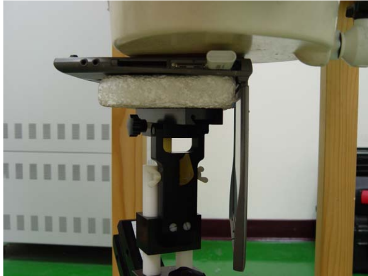
Fig. 9.3 Dell PP03L Notebook Bottom Touch with Horizontal USB Port
