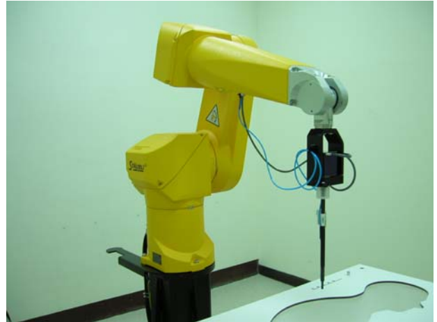
Fig. 5.2 Probe setup on robot
