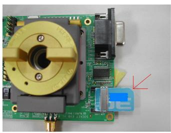
b. Inset the SIM card into the slot.
