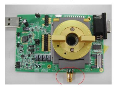
b. Connect the antenna to the adapter.
