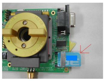
c. Inset the SIM card into the slot.
