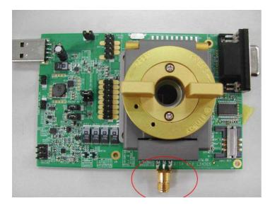
b. Connect the antenna to the adapter.
