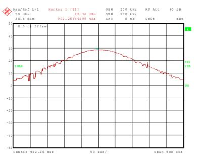
70243\_48.wmf (maximum peak output power at the middle of the assigned frequency band):
