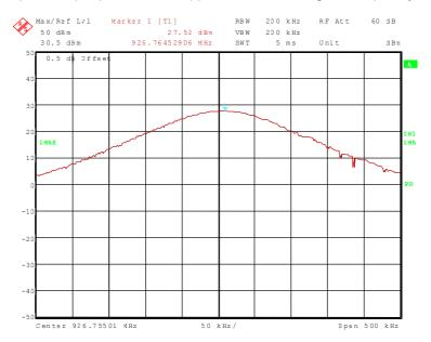
70243\_49.wmf (maximum peak output power at the upper end of the assigned frequency band):
