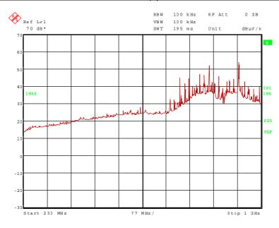
The following frequencies were found outside the restricted bands during the preliminary radiated emission test: 735.250 MHz, 752.750 MHz, 753.750 MHz, 800.750 MHz, 831.250 MHz, 861.750 MHz, 926.250 MHz, 927.250 MHz, 928.250 MHz and 957.750 MHz.
