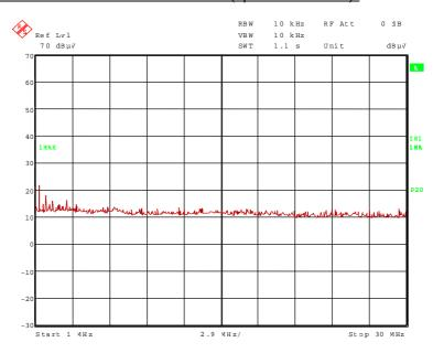
The following frequencies were found during the preliminary radiated emission test: 227.997 kHz, 262.875 kHz, 341.963 kHz, 788.654 kHz and 1.314 MHz.
