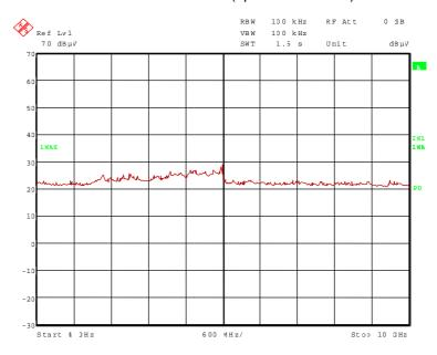
The following frequency was found outside the restricted bands during the preliminary radiated emission test: 1854.500 MHz.
