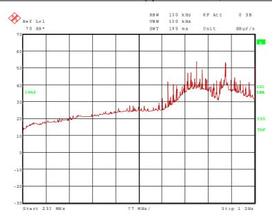
The following frequencies were found outside the restricted bands during the preliminary radiated emission test: 585.250 MHz, 614.750 MHz, 710.750 MHz, 788.250 MHz, 806.750 MHz, 825.250 MHz, 901.750 MHz, 902.750 MHz, 903.150 MHz and 933.250 MHz.
