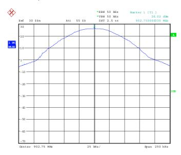
93202\_27.wmf: Maximum peak output power at the middle of the assigned frequency band (operation mode 2):
