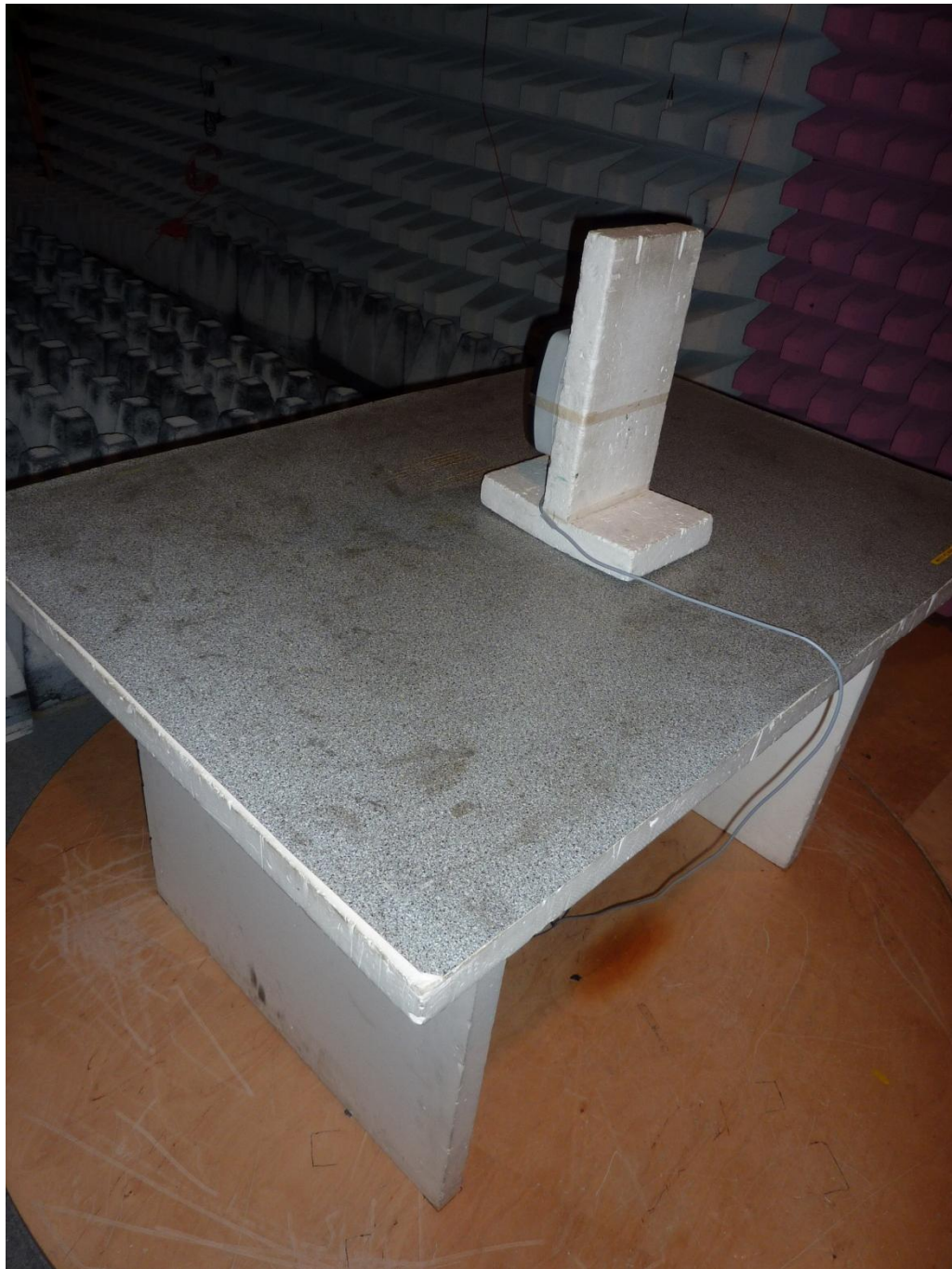
122887_17.JPG: TSU200, test set-up fully anechoic chamber
