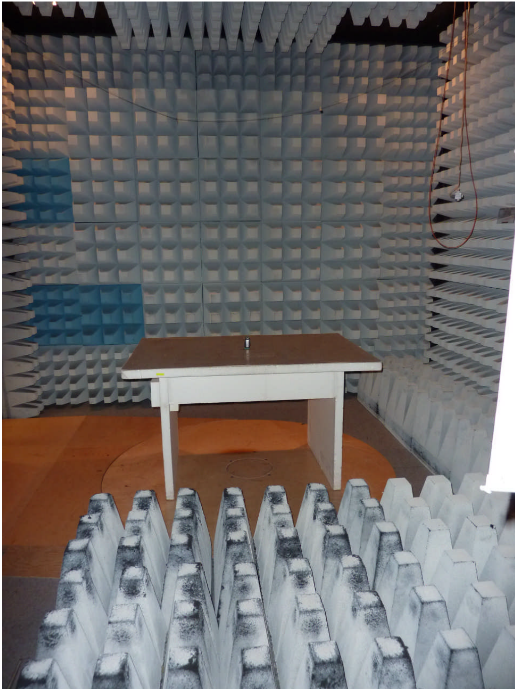
111947_17.JPG: TPU 4030 with housing, test setup fully anechoic chamber (pos. 3)
