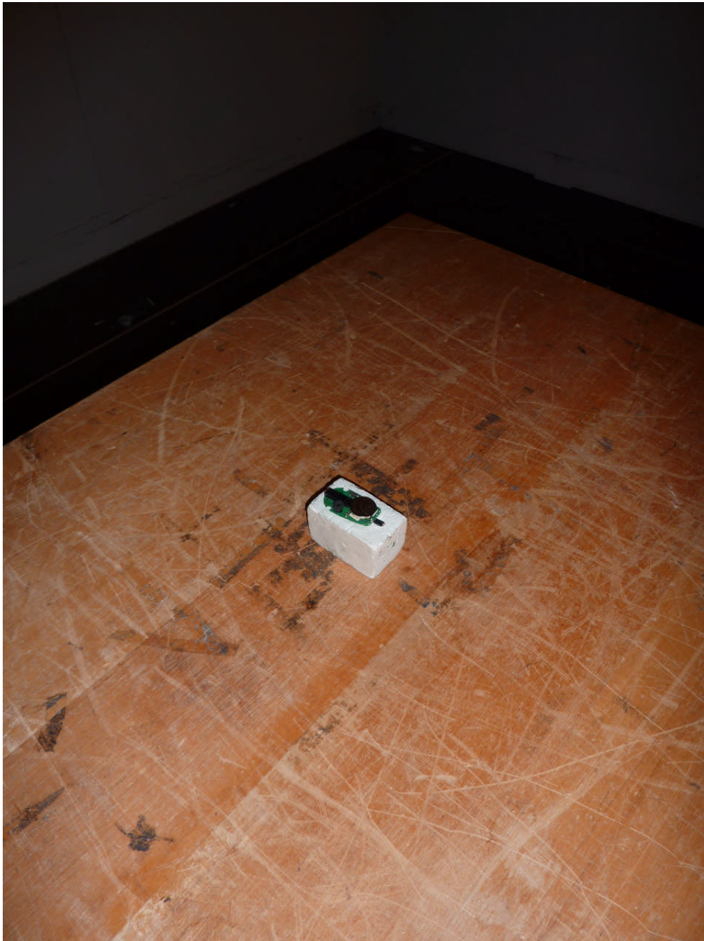
111947_8.JPG: TPU 4030 without housing, test setup open area test site (pos. 1)
