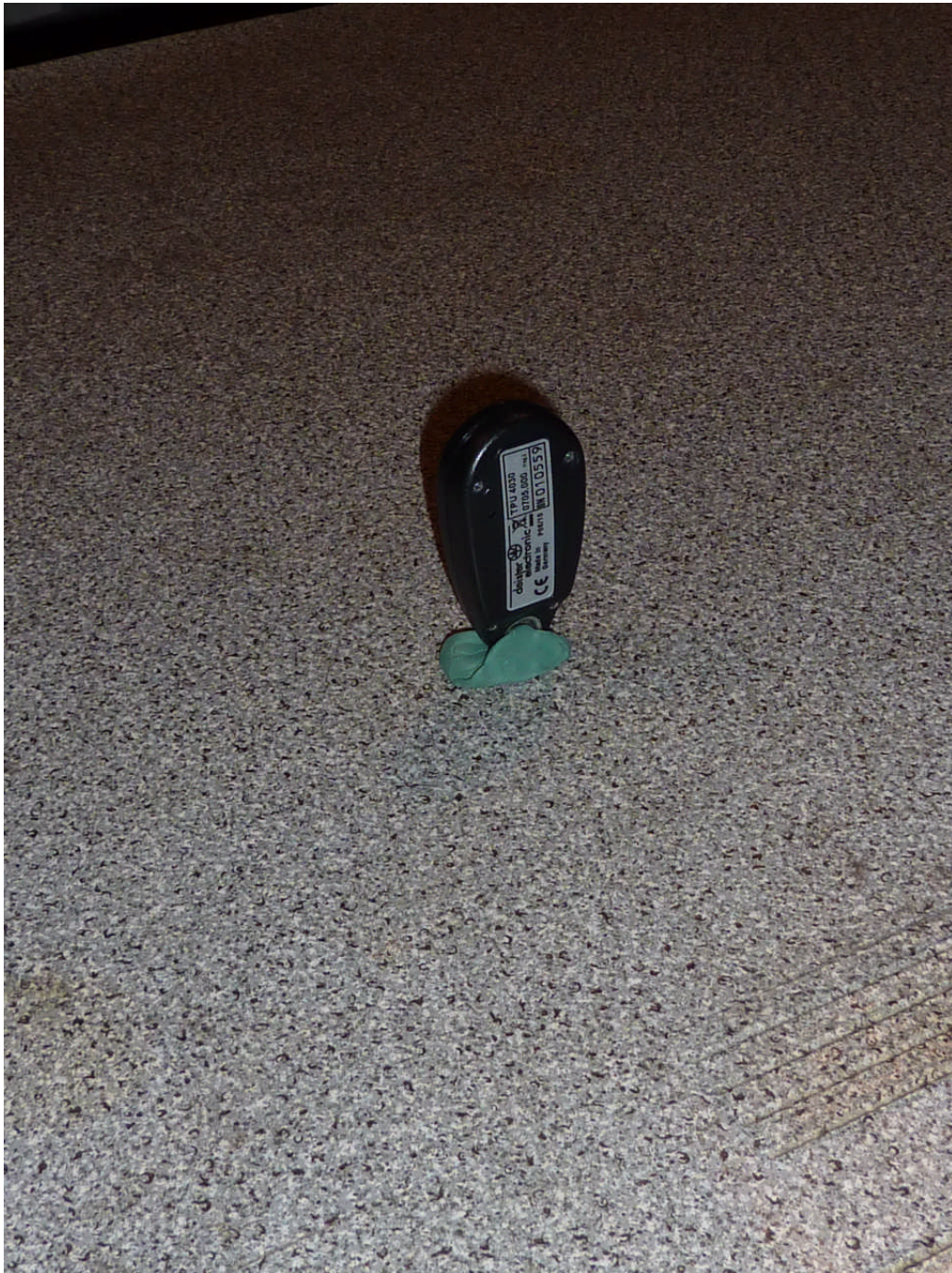
111947_14.JPG: TPU 4030 with housing, test setup fully anechoic chamber (pos. 3)
