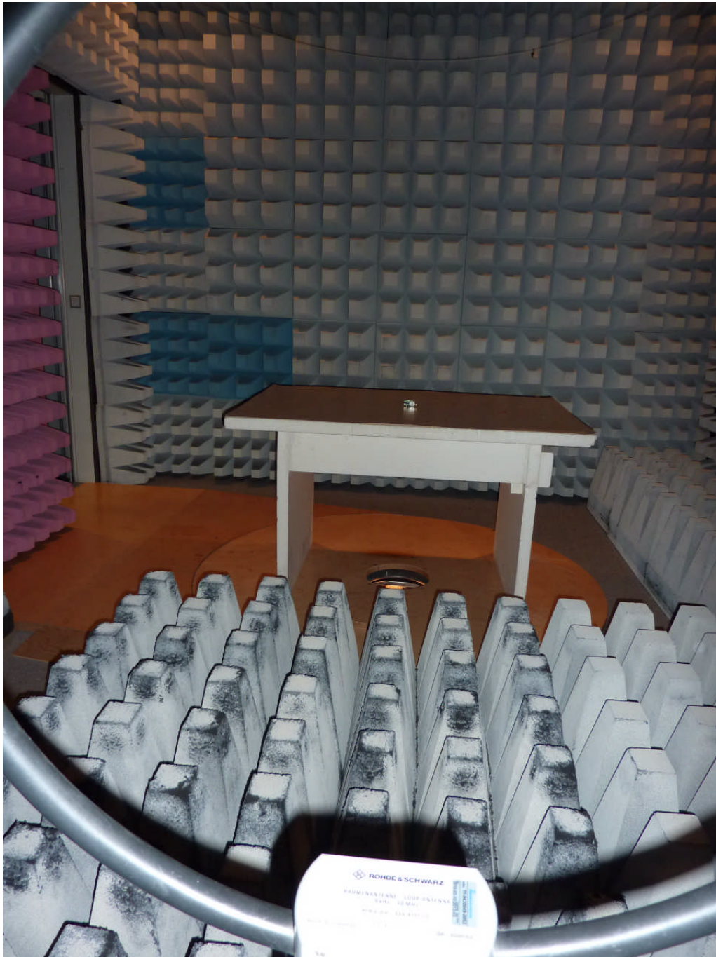
111947_12.JPG: TPU 4030 without housing, test setup fully anechoic chamber (pos. 2)
