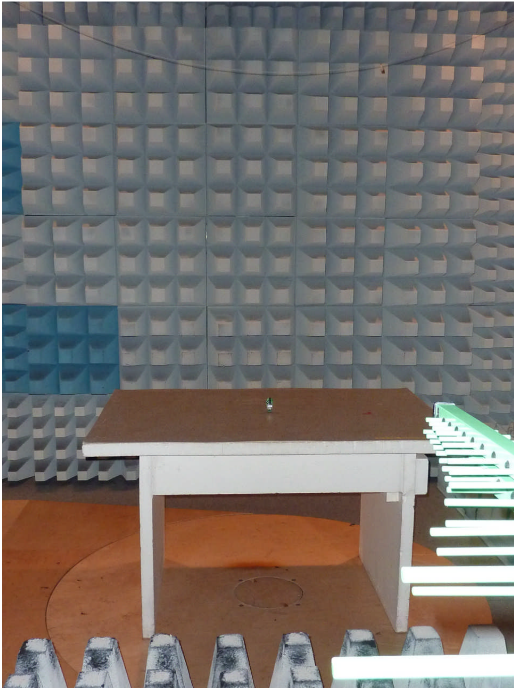
111947_5.JPG: TPU 4030 without housing, test setup fully anechoic chamber (pos. 3)
