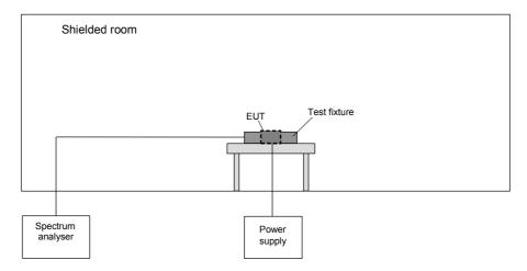
The following procedure will be used for the spectrum mask measurement:
