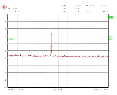
The following emission was found according to FCC 47 CFR Part 15 section 15.209 (a).
