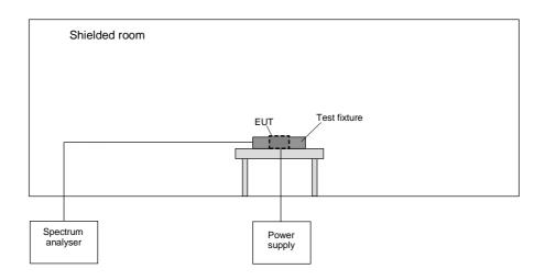
The following procedure will be used for the occupied bandwidth measurement:
