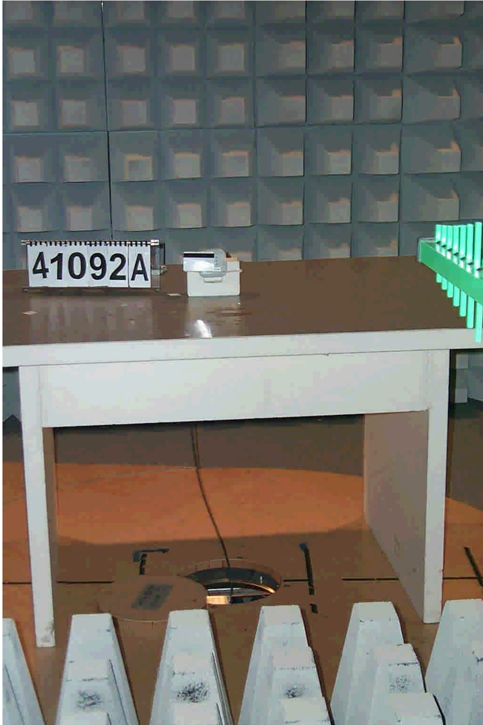
41092A_10.jpg PRM5 / SWH-2100, test set-up fully anechoic chamber
