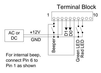
FIGURE 2. Beeper Wiring
