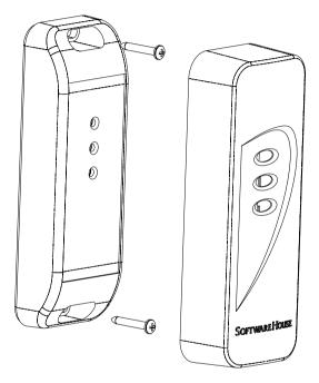
FIGURE 1. Mounting Assembly
