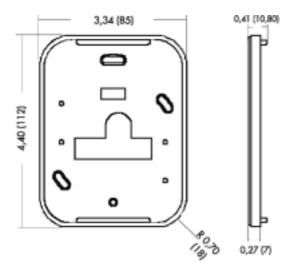
Note: Mounting holes fit a standard US single width electrical box and standard European electrical box hole patterns.
