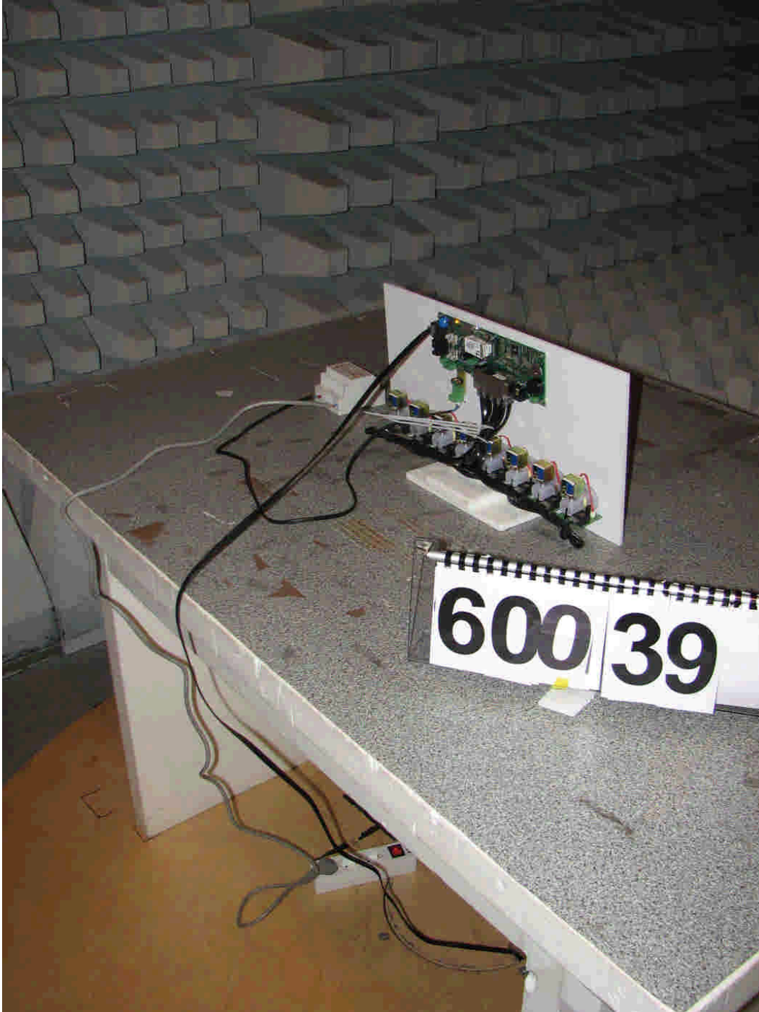
60039_40.jpg ProxSafe mini, test set-up fully anechoic chamber (preliminary test)
