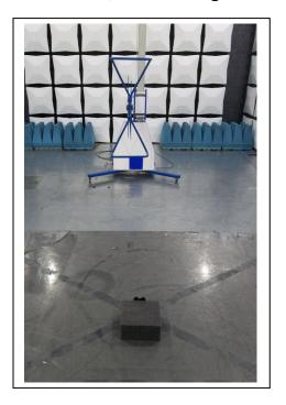
Radiated Spurious, Less Than 30 MHz
