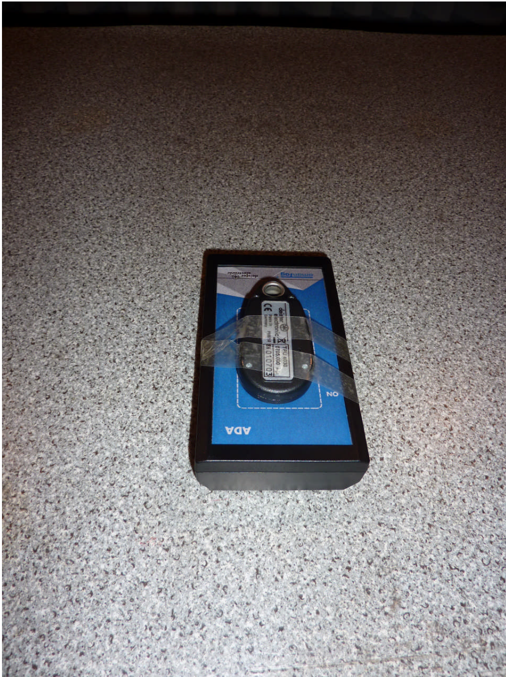
111946_11.JPG: ADA Amantag Deactivator with TAG, test setup fully anechoic chamber (pos. 1)
