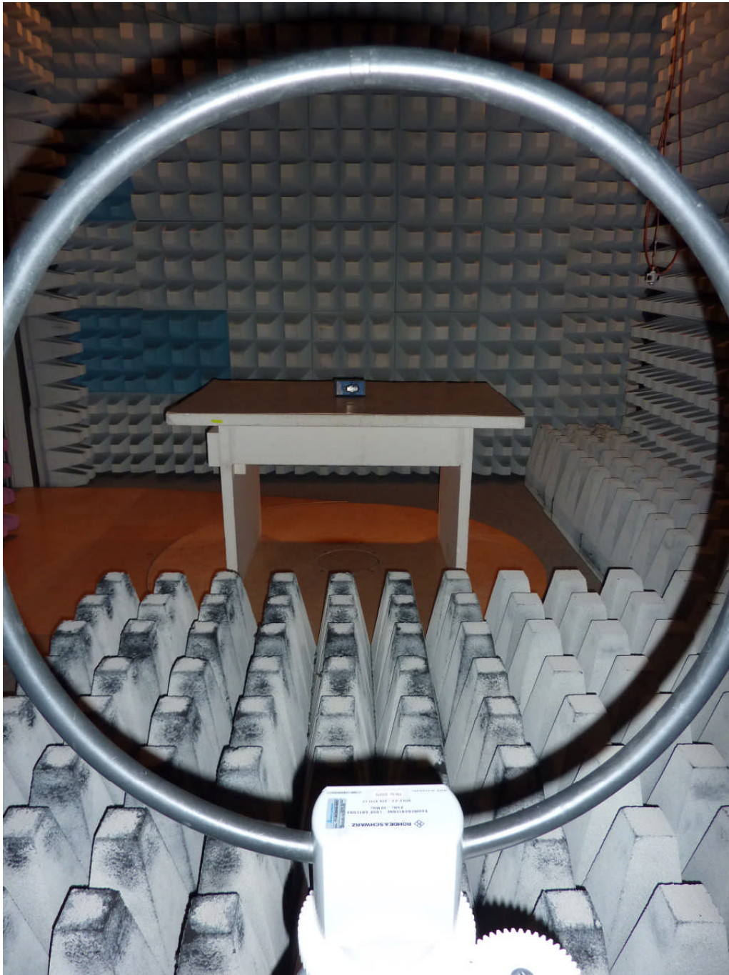
111946_13.JPG: ADA Amantag Deactivator with TAG, test setup fully anechoic chamber (pos. 3)
