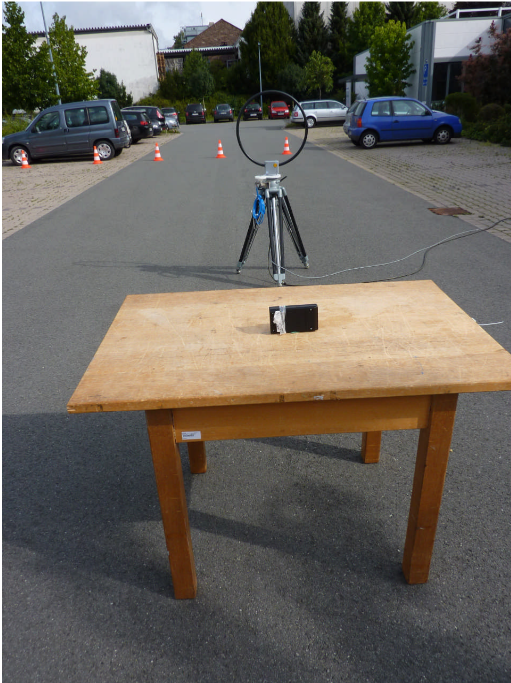
111946_7.JPG: ADA Amantag Deactivator without TAG, test setup outdoor test site
