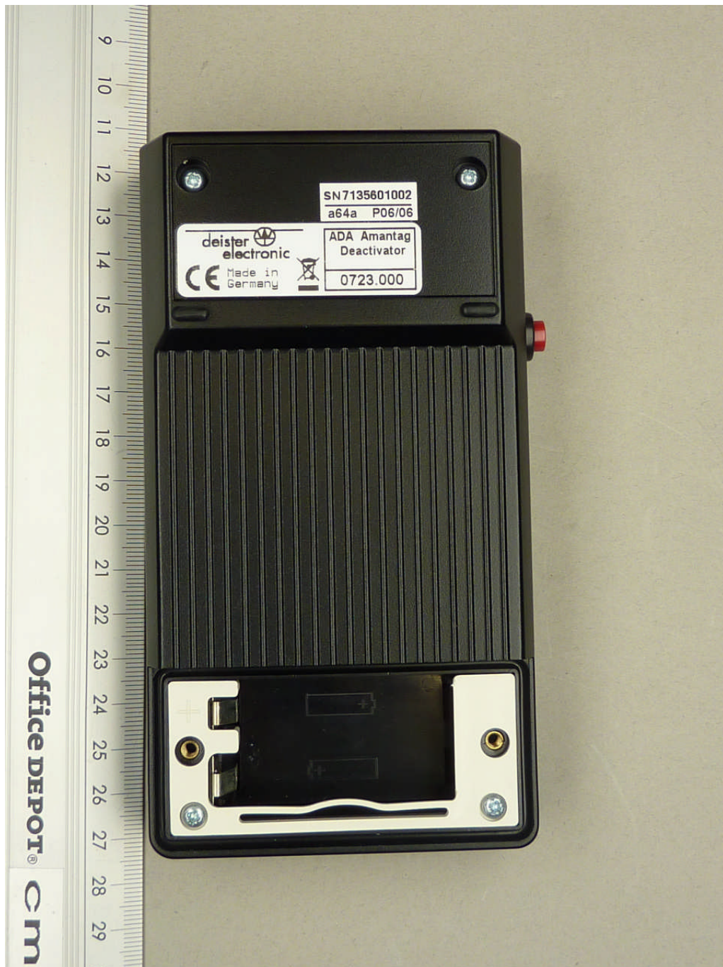
111946_d.JPG: ADA Amantag Deactivator, rear view, battery cover removed
