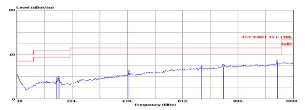
Site no. Limit Env. / Ins. : 3m Chamber : FCC PART 15 C (3M) : 24\*C/56% Data no. : 2 Ant. pol. : HORIZONTAL Engineer : Willis
