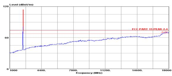
Data no. : 3 Ant. pol. : VERTICAL : RF Chamber : FCC PART 15 PEAK 2.4 : 23\*C/54% Site no. Limit Env. / Ins. Engineer : Willis
