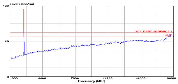
: RF Chamber : FCC PART 15 PEAK 2.4 Data no. : 9 Ant. pol. : VERTICAL Site no. Limit Env. / Ins. : 23\*C/54% Engineer : Willis
