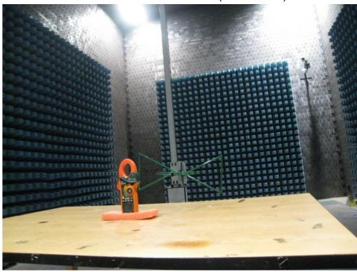
Photo 2 Rear of Radiated Disturbance Test (Below 1GHz)
