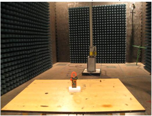
Photo 4 Rear of Radiated Disturbance Test (Above 1GHz)
