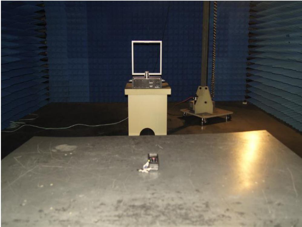
Photograph 2: Set-up for Radiated Spurious Emissions, 30MHz-1GHz
