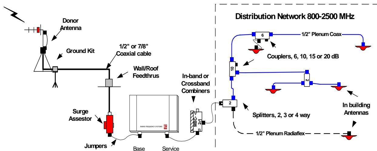
The uplink and downlink amplifiers are broadband to accommodate all the channels in the passband. Differentiation is provided by the duplexing filters. These determine the basic pass band and prevent oscillation between the uplink and downlink by attenuating the opposing link frequencies.
