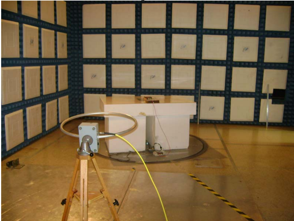
Test Set-up for Radiated Emissions – Horizontal Polarization, External Antenna M190-A2
