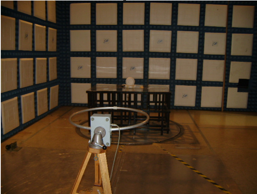
Test Setup for Radiated Emissions – Horizontal Polarization, Integrated Antenna Driver Board
