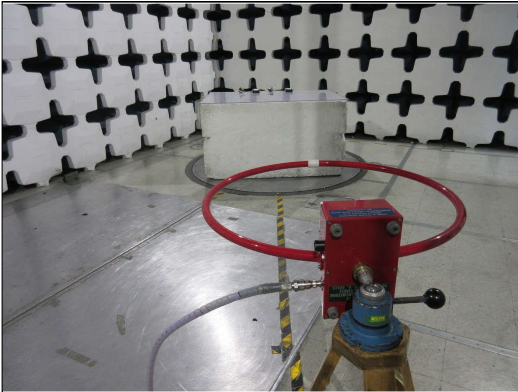
Test Setup for Spurious Radiated Emissions, 10kHz – 30MHz – Antenna Polarization Horizontal
