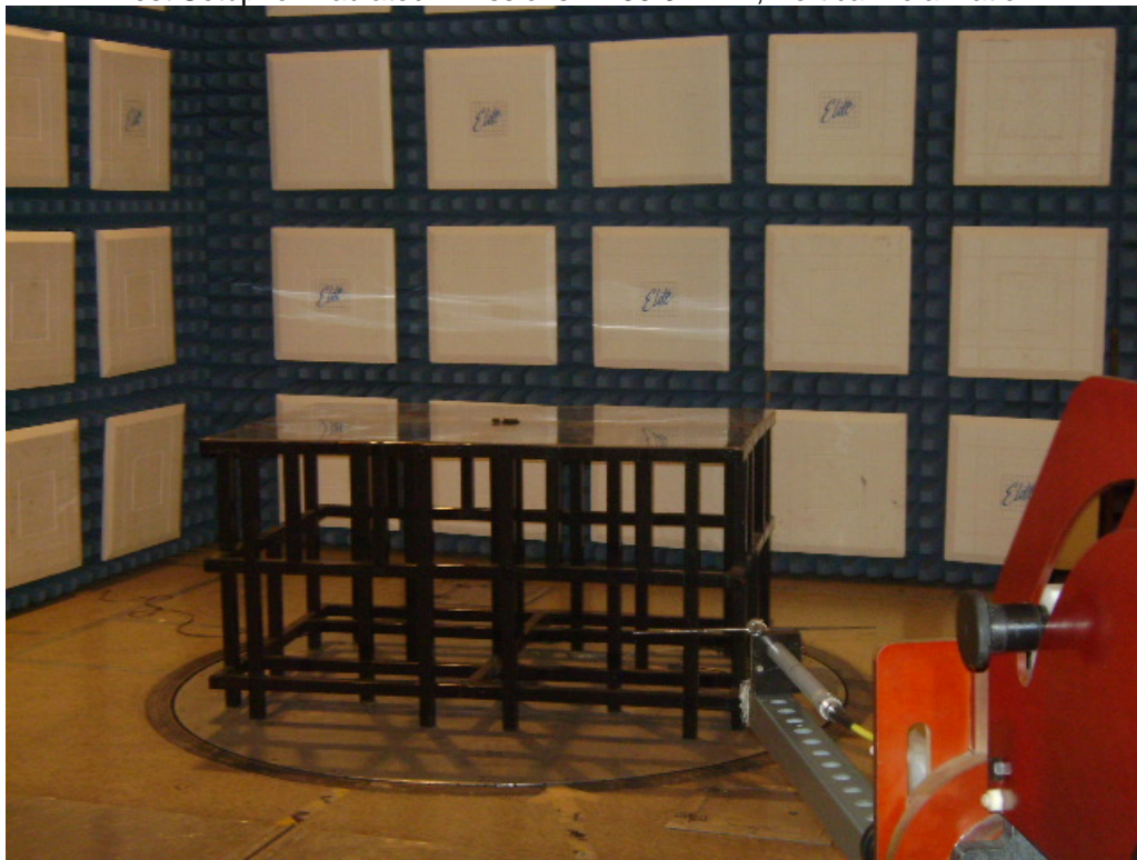
Test Setup for Radiated Emissions – 433.92MHz, Horizontal Polarization
