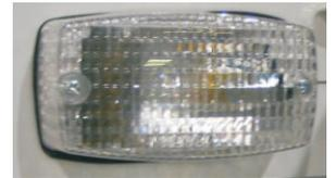
The compartment light can be turned On or Off at anytime by pressing the Light button on FOB. If lights are turned On manually, they will turn Off automatically in 10-minutes.
