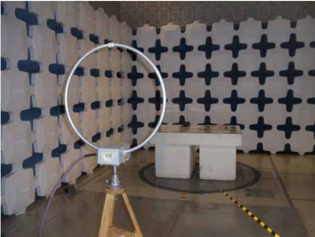
Test Setup for Radiated Emissions, Below 1GHz – Vertical Polarization With M190-A2 external antenna
