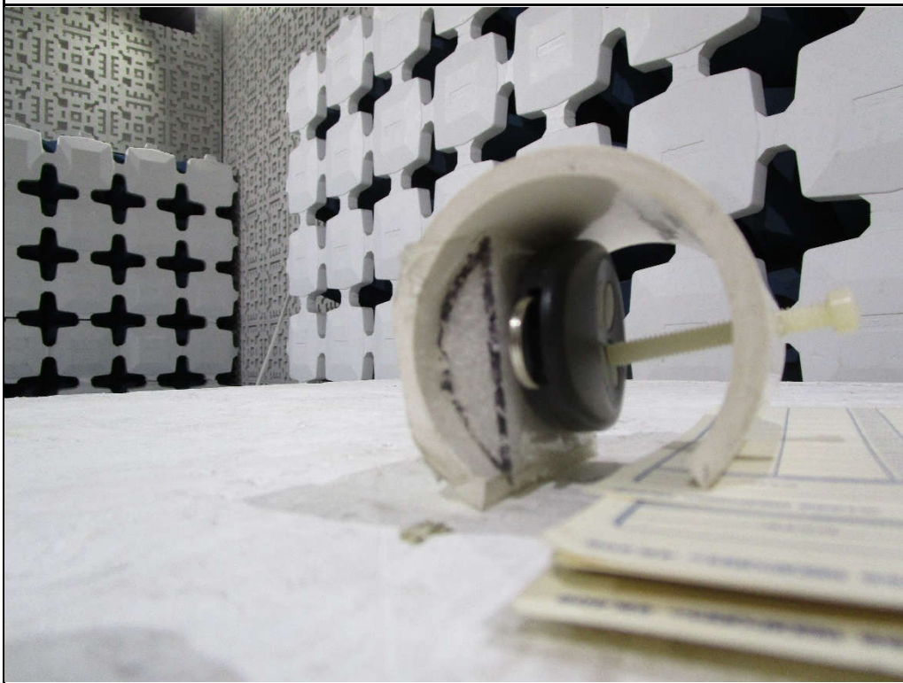
Test Setup for Spurious Radiated Emissions, EUT Oriented in the Y-Axis
