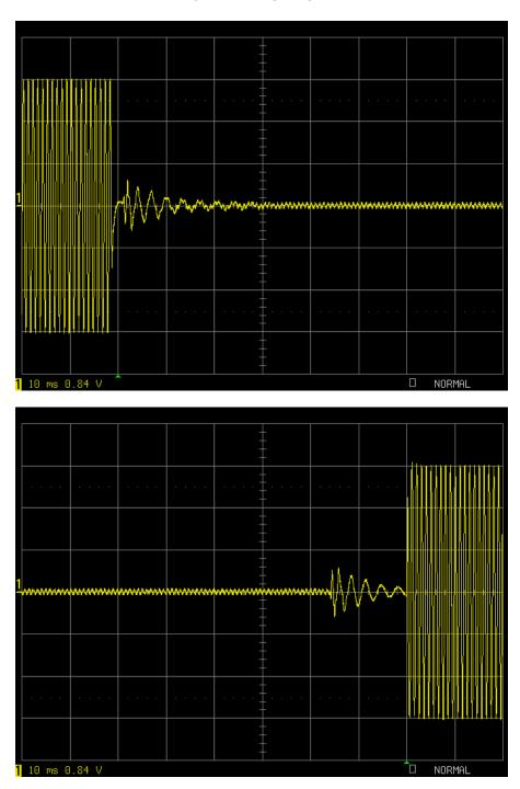
TRANSIENT FREQUENCY RESPONSE 25 kHz - LOW POWER
