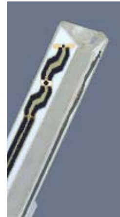
ET3DV6 E-Field Probe
