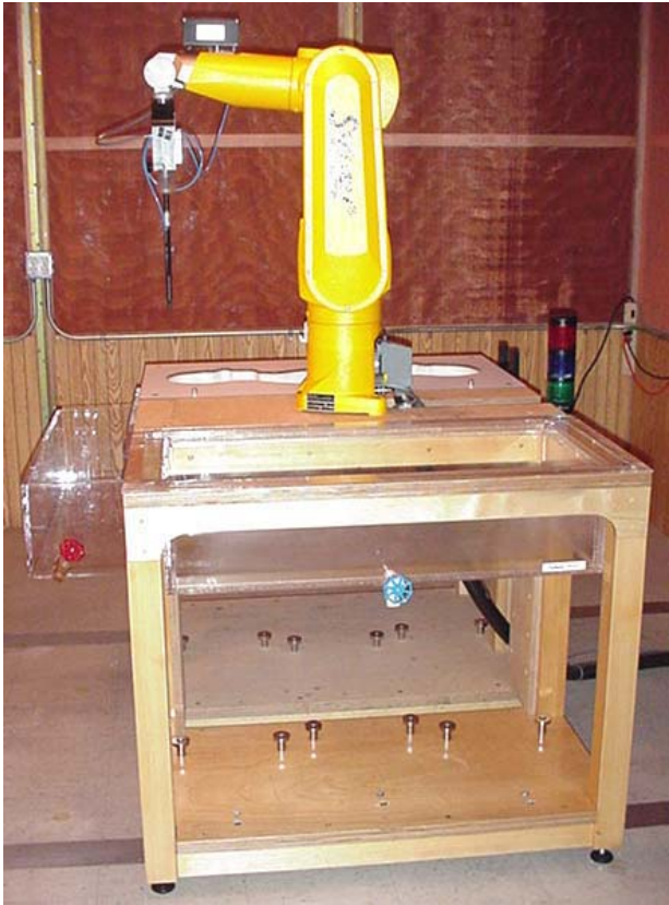
DASY4 SAR Measurement System with validation phantom
