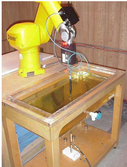
DASY4 SAR System with Plexiglas validation phantom
