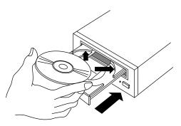
This figure shows in case of Horizontal Installation.
