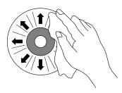
③ Do not write on, or paste paper to the surface of the disc. Should not paste a large or thick label to the outer back surface (the label side) of the disc, or it generates drive vibration due to imbalance of the disc.
