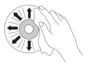
③ Do not write on, or paste paper to the surface of the disc. Should not paste a large or thick label to the outer back surface (the label side) of the disc, or it generates drive vibration due to imbalance of the disc.
