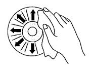
③ Do not write on, or paste paper to the surface of the disc. Should not paste any label to the outer back surface (the label side) of the disc, or it generates drive vibration due to imbalance of the disc.
