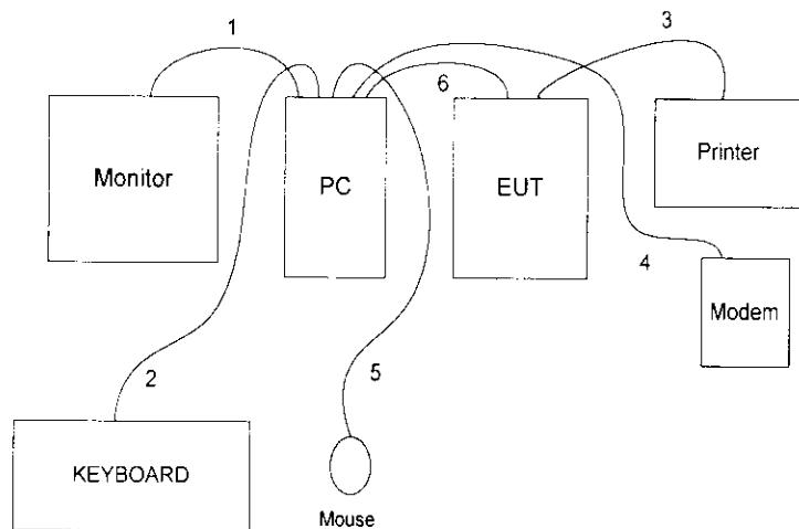
1. The I/O cable is connected from PC to the support device 1.
