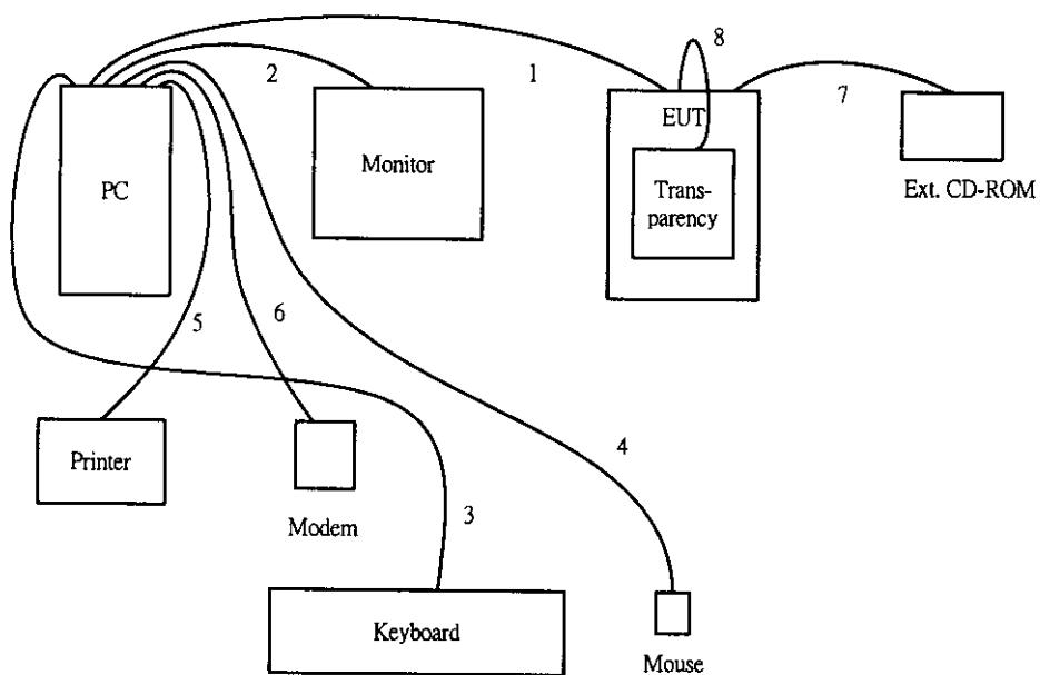
1. The I/O cable is connected from EUT to the support unit 1.
