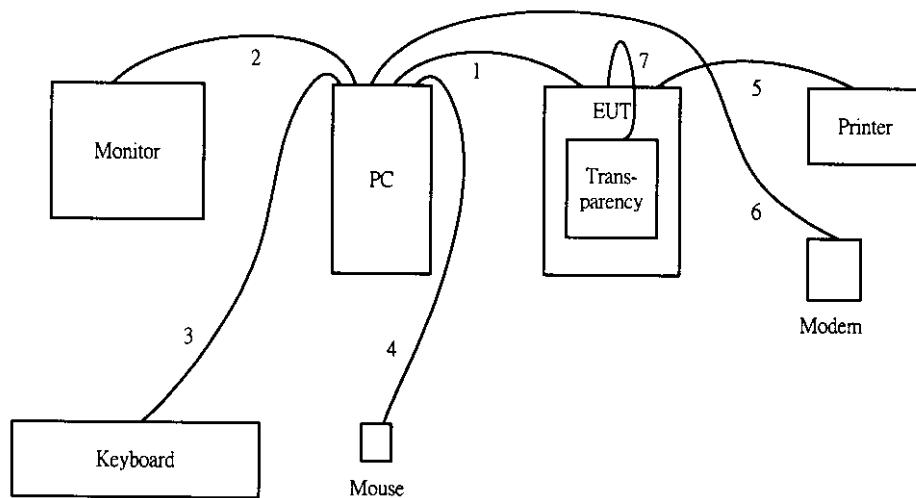
1. The I/O cable is connected from EUT to the support unit 1.
