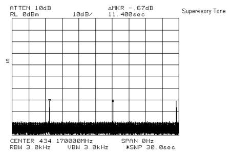
Time between transmissions > 30 x transmission on-time
