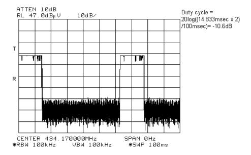
1 Pulse = 14.833 msec, worst case is 2 pulses in 100msec Duty Cycle =  $20\log((2 \times 14.833)/100) = -10.6dB$
