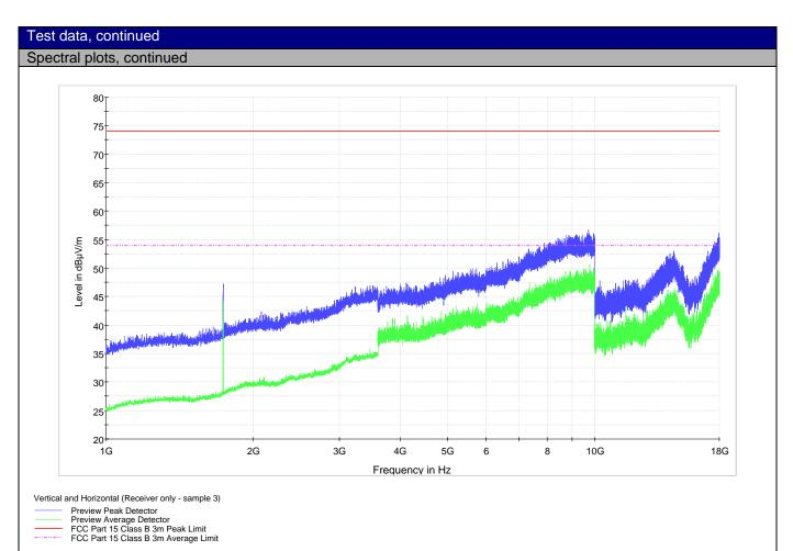
The spectral plot is a summation of a vertical and horizontal scan. The spectral scan has been corrected with transducer factors (i.e. antenna factors, cable loss, amplifier gains, and attenuators) for determination of compliance. Limits have been adjusted to reflect 3 m requirements.
