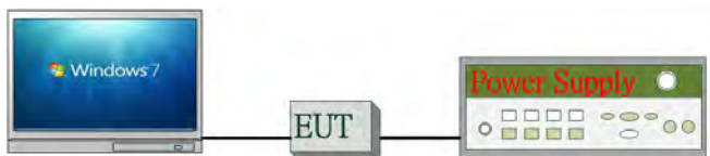
Fig. 2-1 Radiated & Conducted (Antenna Port) Emission Configuration
