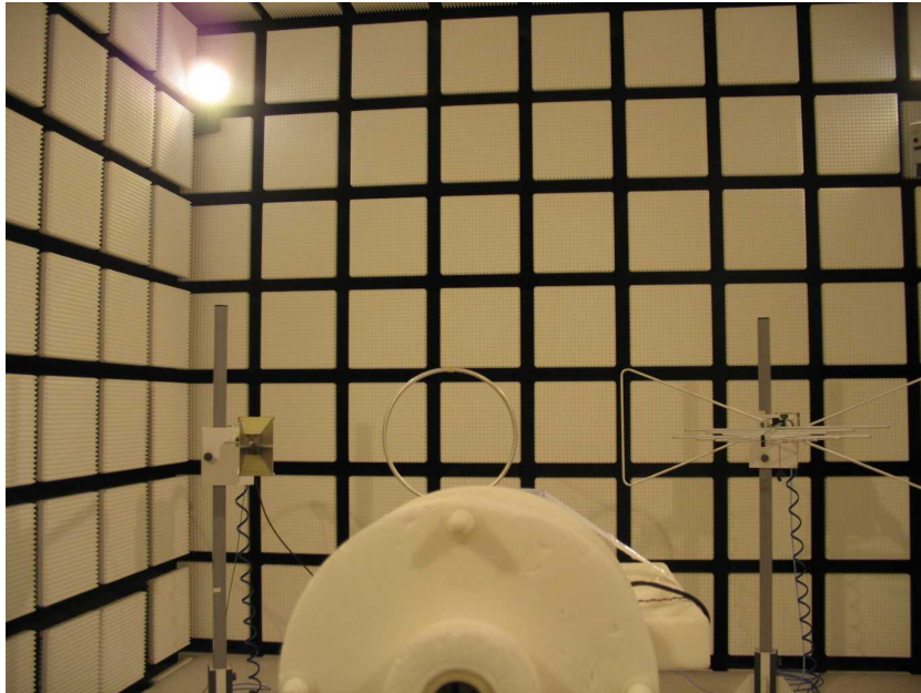
Photo 3: EUT at the anechoic chamber
