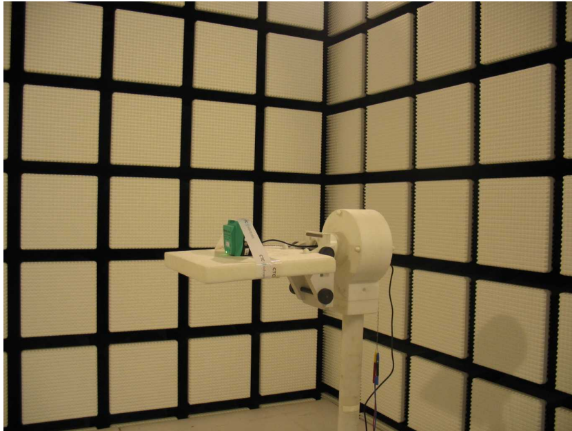
Photo 5: EUT at the anechoic chamber
