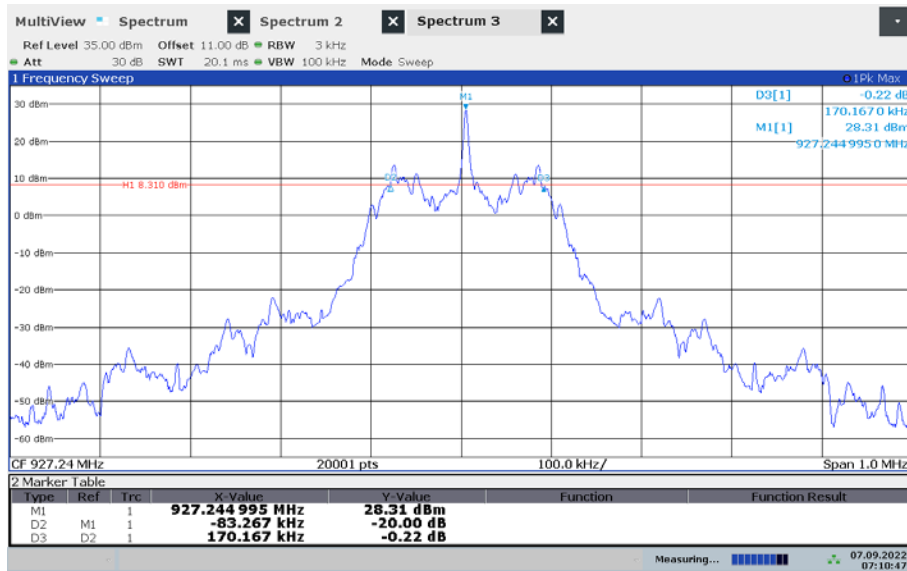
Plot 5: high Channel 20dB bandwidth
