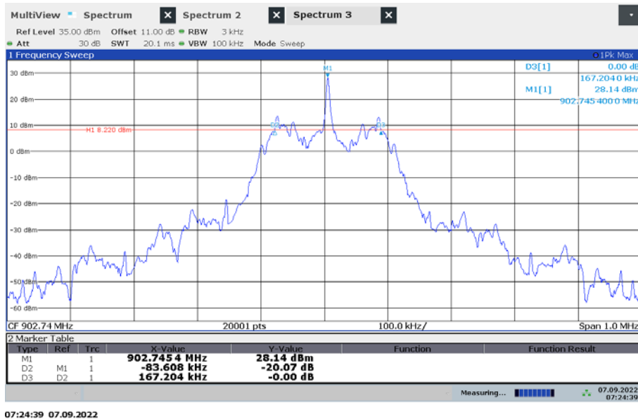
Plot 1: low Channel 20dB bandwidth
