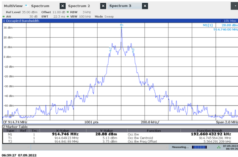
Plot 4: middle Channel 99% bandwidth
