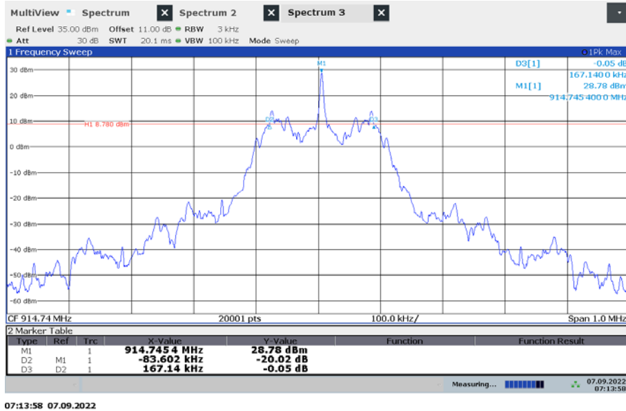
Plot 3: middle Channel 20dB bandwidth
