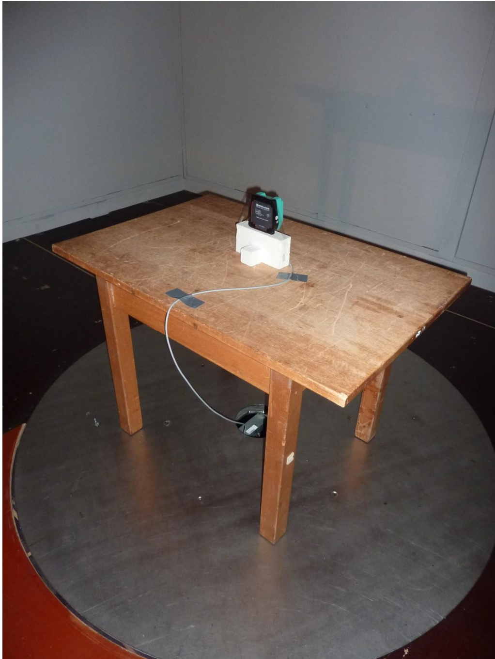
171663_g.JPG: IUHF190V1B, test setup open area test site
