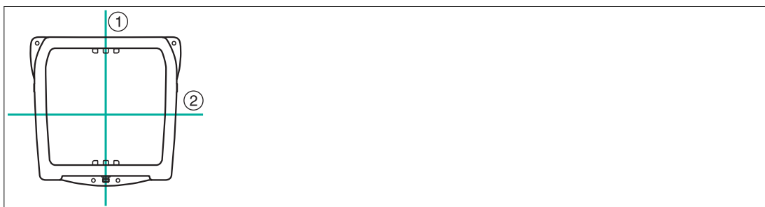
Figure 5.3 ① = Vertical polarization plane ② = Horizontal polarization plane
