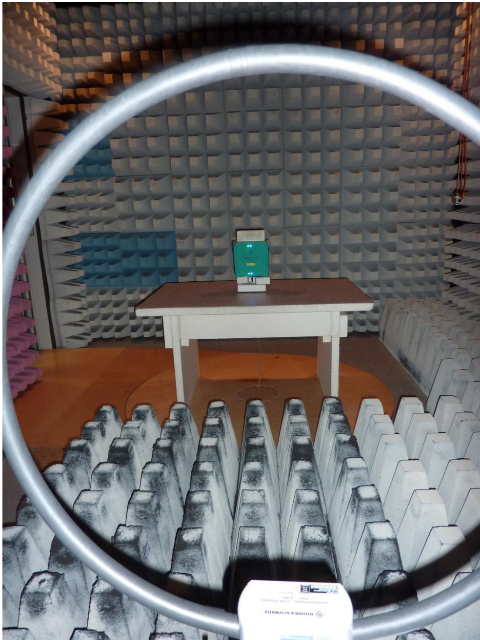
152117_e.JPG: IUH-F192-V1-FR2-02, test setup fully anechoic chamber
