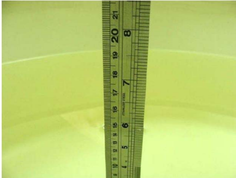
Fig 8.1 Photo of Liquid Height for Body SAR
