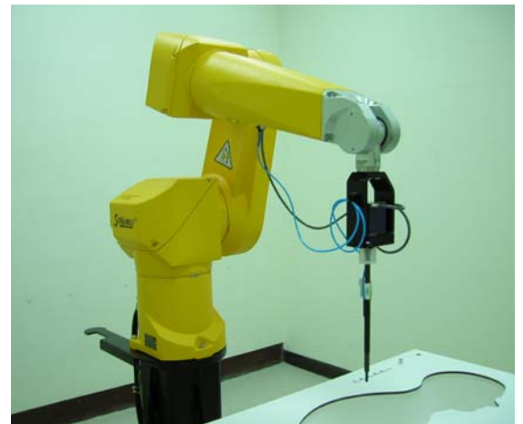
Fig. 5.2 Probe Setup on Robot
