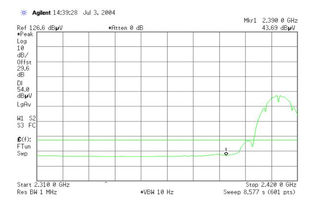
Detector mode: Peak Polarity: Horizontal
